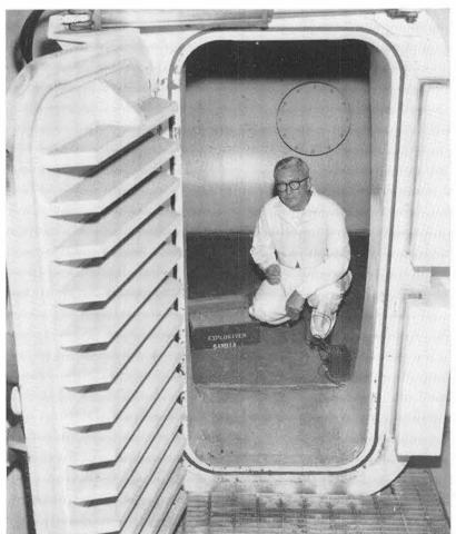
HIGH EXPLOSIVES TECHNICIAN T. K. O'Kelley (8242-1) removes misfired detonator from a charge inside one of the Livermore Laboratory firing chambers. The detonator will eventually be destroyed in the explosives incinerator along with other faulty explosive devices.
